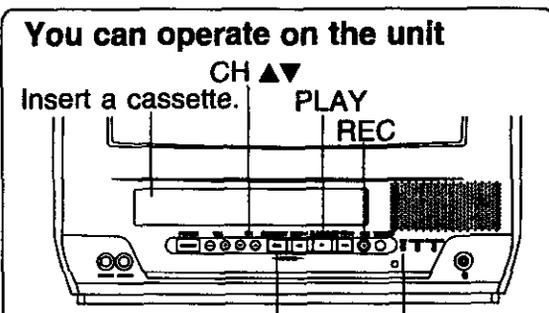
■ Press to stop and/or eject tape. REC Indicator
