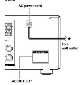
\* The configuration, shape, and number of AC outlets vary according to the model and country to which the receiver is shipped.
