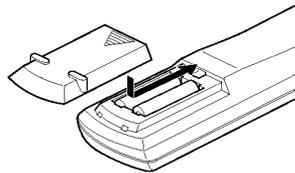
If the range or effectiveness of the remote control decreases, replace the batteries. Use two R6P (SUM-3)/AA (15F) type dry-cell batteries.
