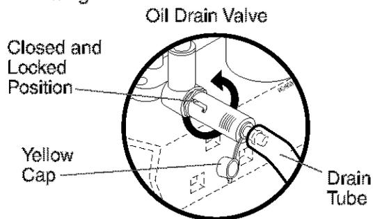
3. Unlock drain valve by pushing inward slightly and turning counterclockwise.
