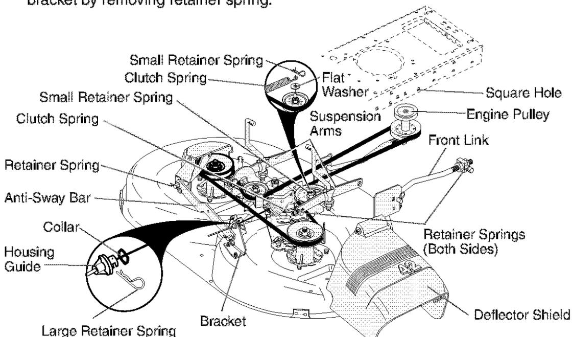
2. Slide mower under tractor with deflector shield to right side of tractor.
