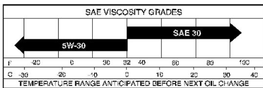
**NOTE:** Although multi-viscosity oils (5W30, 10W30 etc.) improve starting in cold weather, the oils will result in increased oil consumption when used above 32°F. Check your engine oil level more frequently to avoid possible engine damage from running low on oil.
