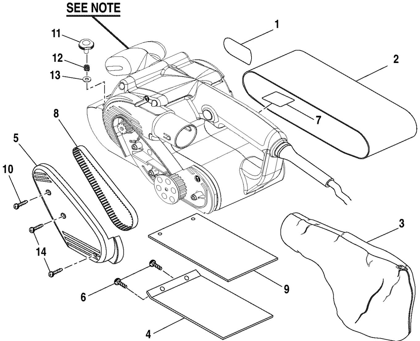
**Note:** The assembly shown represents an important part of the double insulated system. To avoid the possibility of alteration or damage to the system, service should be performed by your nearest Sears repair center. Contact your nearest Sears retail store for service center information.
