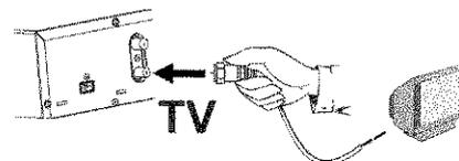
**3** Connect the **S-VIDEO OUT / AUDIO L/R OUT** jacks or **VIDEO (CVBS) OUT / AUDIO L/R OUT** with the corresponding input jacks of the TV.
