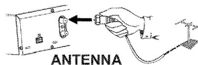
**2** Insert one end of the supplied antenna cable into the **TV OUT** jack at the back of the DVD Recorder and the other end into the antenna input jack at the back of the TV.
