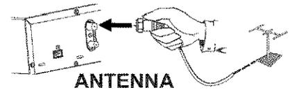
**2** Insert one end of the supplied antenna cable into the **TV OUT** jack at the back of the DVD Recorder and the other end into the antenna input jack at the back of the TV.
