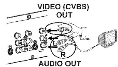
**4** Use an audio (cinch) cable and plug one end into the red/white cinch jack **AUDIO L/R OUT** at the back of the DVD Recorder (under to **Video in**) and the other into the corresponding red/white audio input jack of the TV (usually called Audio in', 'AV in'. See your TV's instruction manual).
