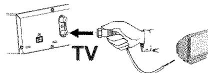
**3** Use a Component Video (Y PB PR) cable and connect one end to the red, blue, green **COMPONENT VIDEO OUT** jacks at the back of the DVD Recorder and the other end to the Component Video In jacks of the TV.
