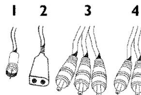
**1** Remove the antenna cable plug from your TV. Insert it into the **ANTENNA IN** jack at the back of the DVD recorder.
