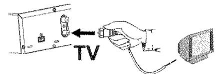
**3** Use a video (CVBS) cable and plug one end into the yellow jack **VIDEO (CVBS) OUT** at the back of the DVD Recorder and the other end into the Video In jack (usually yellow) of the TV (usually called Video in or AV in. See your TV's instruction manual).
