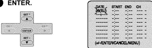
**4** Set the start time, end time, channel and tape speed as in step 3.
