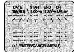
**6** Press **TIMER REC**. The timer symbol (⏺) will appear on the display and the VCR stands by for recording.
