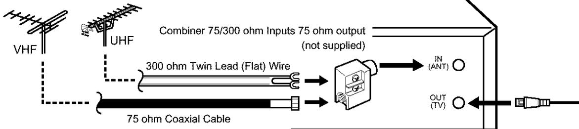
**Note:** If both VHF and UHF antennas have 300 ohm twin lead (flat) wires, use a combiner having two 300 ohm inputs and one 75 ohm output.
