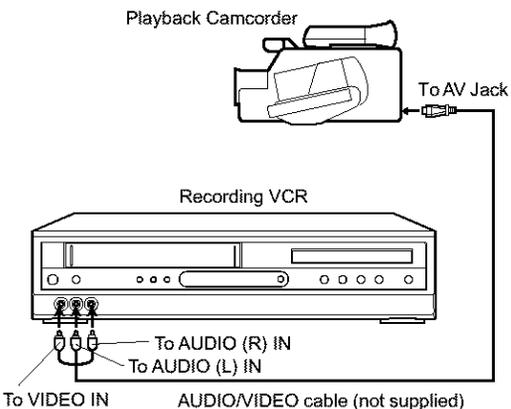
For duplicating a previously recorded tape from a camcorder, follow the camcorder manufacturer's instructions. A typical camcorder dubbing hookup is shown above.
