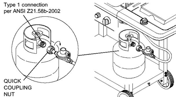
**CAUTION:** When the appliance is not in use, the gas must be turned off at the supply tank.
