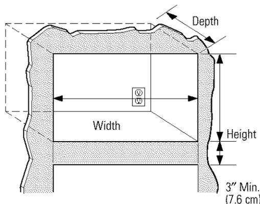
On 27" (68.6 cm) models, allow 1" (2.5 cm) at the top,  $\frac{1}{16}$ " (1.75 cm) on the sides and 1 $\frac{3}{8}$ " (3.5 cm) at the bottom for overlap of the Trim Frame over the edges of the cutout.
