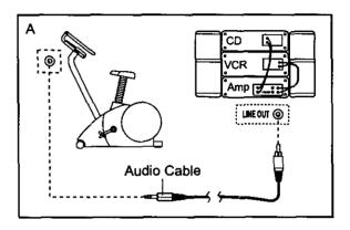
B. Plug one end of a 1/8" to RCA stereo audio cable (available at electronics stores) into the jack beneath the console. Plug the other end of the cable into an RCA Y-adapter (available at electronics stores). Next, remove the wire that is currently plugged into the LINE OUT jack on your stereo and plug the wire into the unused side of the Y-adapter. Plug the Yadapter into the LINE OUT jack on your stereo.
