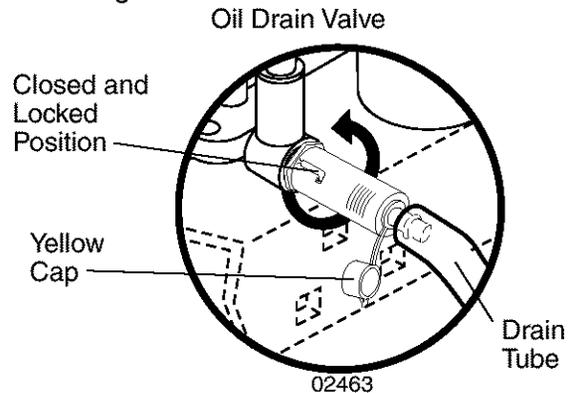
3. Unlock drain valve by pushing inward slightly and turning counterclockwise.
