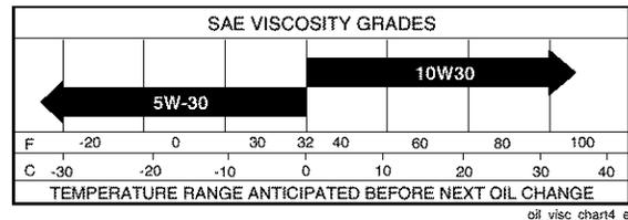
Change the oil after every 50 hours of operation or at least once a year if the tractor is not used for 50 hours in one year. Check the crankcase oil level before starting the engine and after each eight (8) hours of operation.
