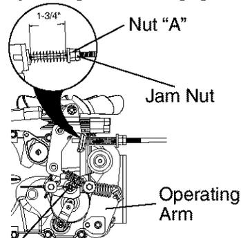
Do not touch this nut. If further brake adjustment is necessary contact a Sears or other qualified service center.
