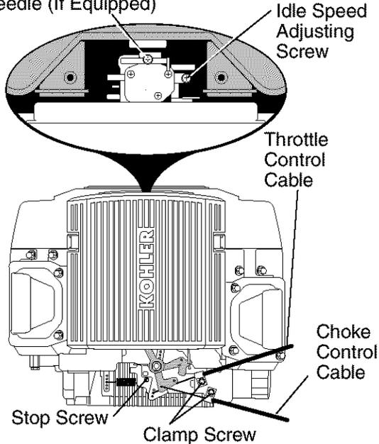
control (located on dash panel) to full choke position.
