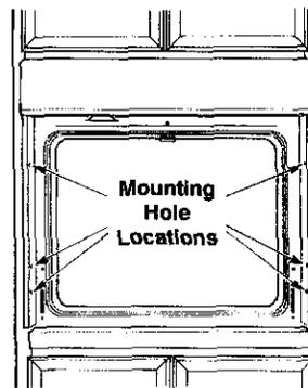
The screws must be a minimum of 1/4" from the front of the cutout.
