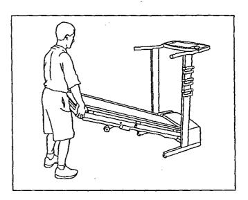
Next, hold the upper end of the treadmill with your right hand as shown. Using your left hand, pull the treadmill knob to the left. Pivot the treadmill until the lock pin is aligned with the hole in the side of the treadmill frame (refer to the inset drawing).
