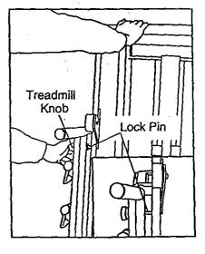
Slowly release the knob. Make sure that the lock pin is inserted into the hole in the treadmill frame.
