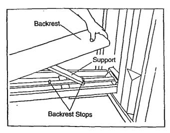
To adjust the backrest to the level position. first raise the backrest slightly. Pivot the end of the support in the direction shown by the arrow. Lower the backrest
