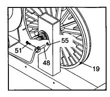
for clarity). Slide the Reed Switch slightly toward or away from the Magnet. Make sure that the Magnet will not hit the Reed Switch. Retighten the Screw. Turn the Pulley (19) for a moment. Repeat until the console displays correct feedback. When the Reed Switch is correctly adjusted, re-attach the Left Side Shield (11).
