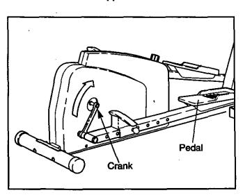
To dismount the REBEL, allow the pedals to slowly come to a stop. CAUTION: The REBEL does not have a freewheel; the pedals will continue to move until the flywheel stops. When the pedals are stationary, step off the highest pedal first. Then, step off the lowest pedal.
