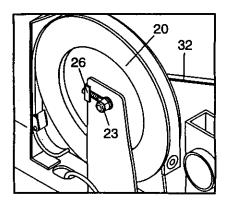
counterclockwise. Make sure that the Flywheel is straight and retighten the M8 Flange Nuts (23). When the Drive Belt is properly adjusted, re-attach the Side Shields.
