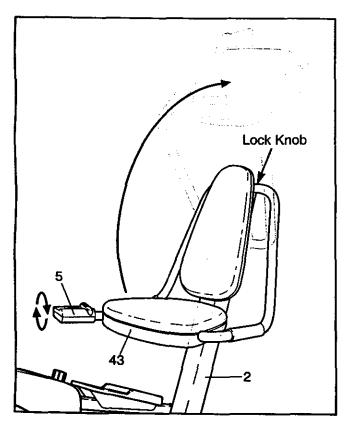
To switch from elliptical crosstrainer to recumbent bike, unscrew the Lock Knob (81, not visible). Fold the Seat (43) down and turn the Console (5) so it is visible when you are sitting on the Seat.
