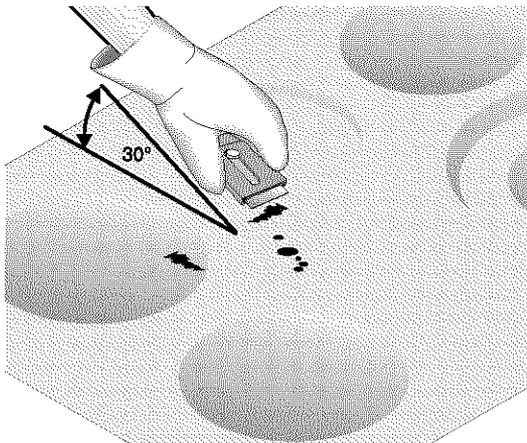
If soils remain, carefully scrape soils with a metal razor blade scraper, holding scraper at a 30 degree angle to the surface. Remove loosened soils with cooktop cleaner and buff surface clean.
