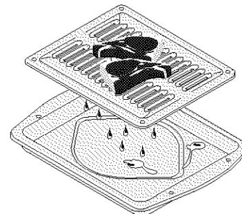
The broiler pan and the insert allows grease to drain and be kept away from the high heat of the broiler. **DO NOT** use the pan without the insert. **DO NOT** cover the insert with foil; the exposed grease could ignite.
