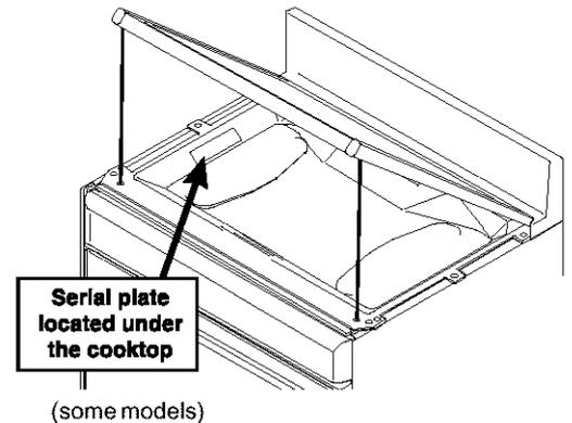
The product serial plate will provide you both the model number and serial number for your range. You can find the serial plate on your range at one of the locations illustrated above.
