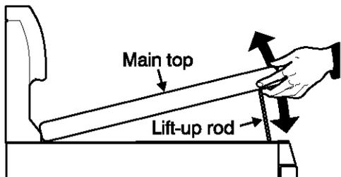
**CAUTION** When lowering the lift-up range top, grasp the sides with finger-tips only. Be careful not to pinch fingers. **DO NOT** drop or bend the range top when raising or lowering. This could damage the surface.
