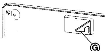
Rotate microwave hood up towards cabinet. Push microwave hood against mounting plate until locking latch **G** snaps into microwave hood.
