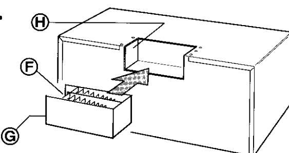
Slide air deflector back into cabinet as far as it will go. Check that deflector vanes ⑤ face the top of the cabinet and that the small exhaust ports ⑥ ⑦ face each other.
