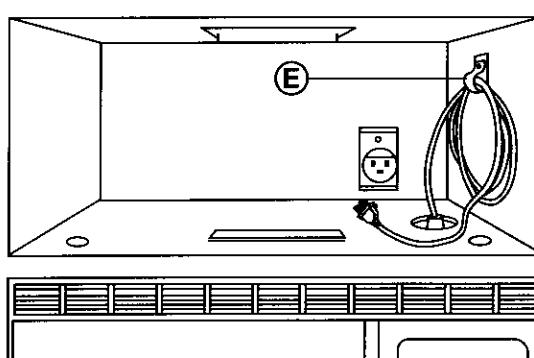
Coil power supply cord through clamp ⑧. Secure clamp to cabinet side wall with dark colored screw.
