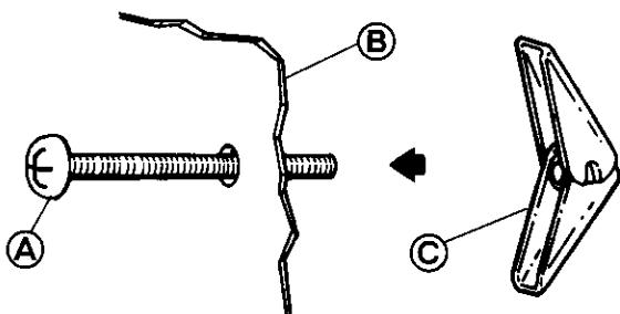
Insert 1/4" x 3" toggle bolts **A** through holes in mounting plate **B** that match the location of the 3/4" holes in the drywall.
