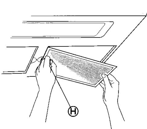
Grasp aluminum filter screen by the tab **H** and insert tab end of filter into cabinet opening. Slide towards the center of microwave hood. Insert other end of filter into opening and slide entire filter towards the side of the microwave hood until filter is securely in position. Repeat for other filter.
