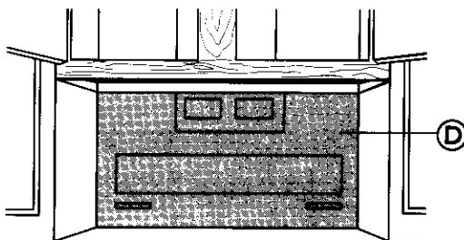
Position mounting plate **D** on the wall. Push toggle bolts **A** and nuts **C** through the drywall **E**.
