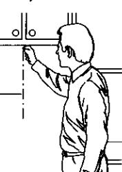
Line up paper wall template centerline with centerline on wall. Tape or tack wall template to wall. Top of template must be located a minimum of 66" from floor.
