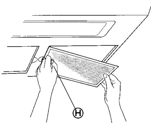
Grasp aluminum filter screen by the tab **H** and insert tab end of filter into cabinet opening. Slide towards the center of microwave hood. Insert other end of filter into opening and slide entire filter towards the side of the microwave hood until filter is securely in position. Repeat for other filter.
