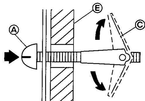
Finger tighten the toggle bolts **A** to make sure toggle nuts **C** have opened against drywall **E**.
