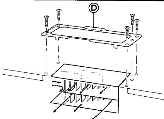
Reattach damper plate ④ with five screws.
