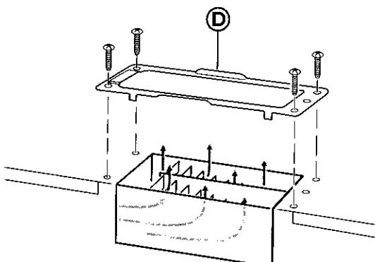
Reattach damper plate ④ with four screws at each corner of the damper plate. Save bright-colored tapping screw for use later to attach damper assembly.
