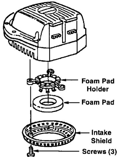
6. Replace foam pad holder on blower with the tabs away from the blower. Reinstall foam pad under the tabs of the holder.
