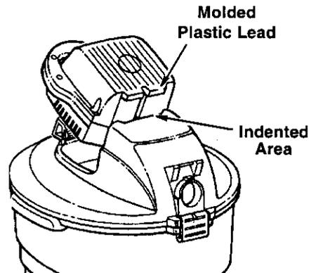
3. Rotate the detachable blower down until the travel of the unit stops.
