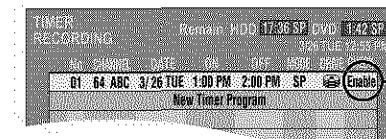
Displayed if the recording can fit in the remaining space on the HDD or disc.
