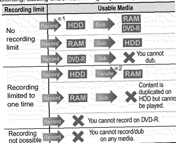
\*1Turning "DVD-R compatible Rec" to "On" from the Setup menu allows dubbing to a DVD-R using the high speed mode after a recording has been saved to the HDD. (→page 44)
