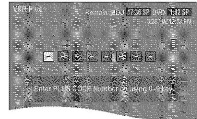
**2 Press the numbered buttons to enter the VCR Plus+ code.**
