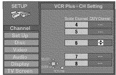
**5 Press [▲, ▼] to select the channel corresponding to the guide channel and press [◀].**
