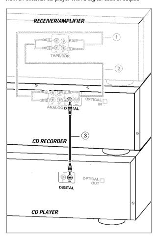
**1** For external recording, connect the cord ③ between the DIGITAL IN-jack on the set and the DIGITAL OUT-jack of an external CD player.
