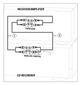
Use the audio cords supplied. Connect the red plugs to the R jacks, and the white plugs to the L jacks.
