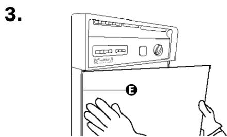
3. Insert one side of door panel, with desired color facing out, into one side of door frame **E**.
