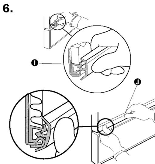
6. Snap one end of retainer into channel as shown **I**. Push inward while sliding thumb along full length of retainer **I**.
