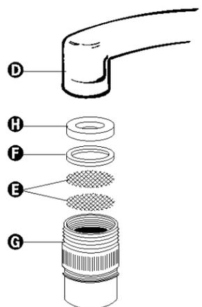
Insert both screens **E**, the thin washer **F** and then the thick washer **H** into faucet adapter **G**. Attach adapter onto end of faucet **D**. Both washers need to be used.
