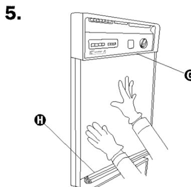
5. Push in on door panel near the top and slide panel and spacer up inside bottom of control console **G**, allowing panel to rest on channel **H** at bottom of door.
