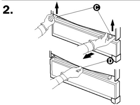
2. Lift door panel at outer edges **C**. Use one hand to bow bottom of panel **D**. Remove panel. Do Not remove spacer.
