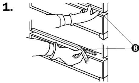
1. Insert finger under one end of retainer **B** and pull retainer towards you in a peeling action. Set retainer aside.
