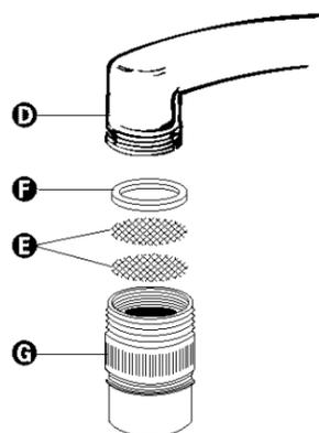
Insert both screens **E** and thin washer **F** into faucet adapter **G**. Attach adapter onto end of faucet **D**. The thick washer is not used.
