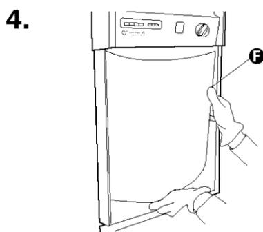
4. Bow door panel and insert other side of door panel into door frame **F**.
