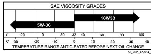
Change the oil after every 50 hours of operation or at least once a year if the tractor is not used for 50 hours in one year. Check the crankcase oil level before starting the engine and after each eight (8) hours of operation.
