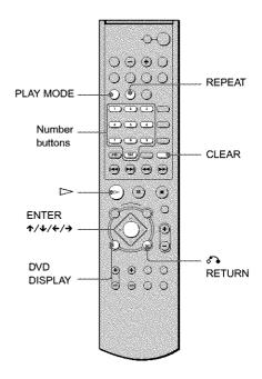
In stop mode, press PLAY MODE repeatedly until "PROGRAM" appears on the front panel display.
