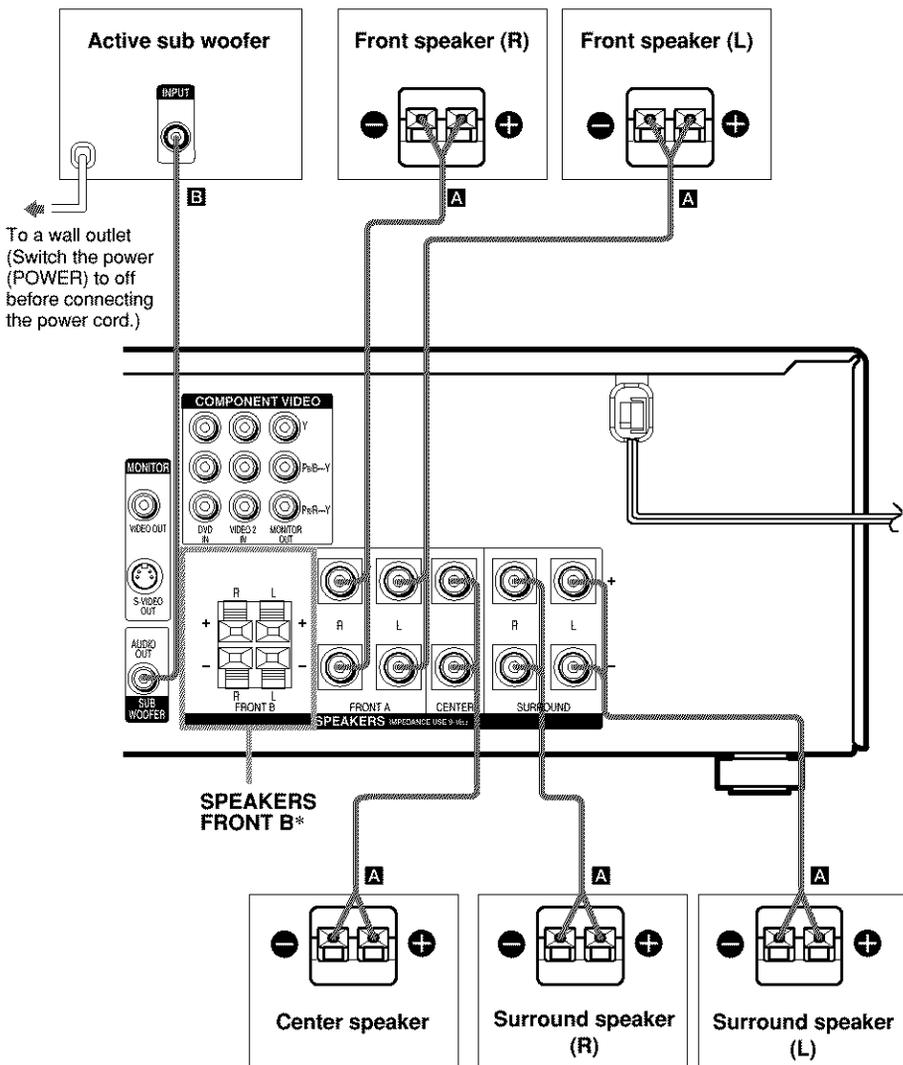
\* If you have an additional front speaker system, connect them to the SPEAKERS FRONT B terminals. You can select the front speakers you want to use with the SPEAKERS (OFF/A/B/A+B) button (page 23).
