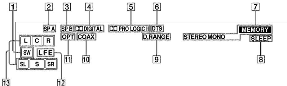
**1 SW:** Lights up when sub woofer selection is set to “YES” (page 19) and the audio signal is output from the SUB WOOFER jacks.
