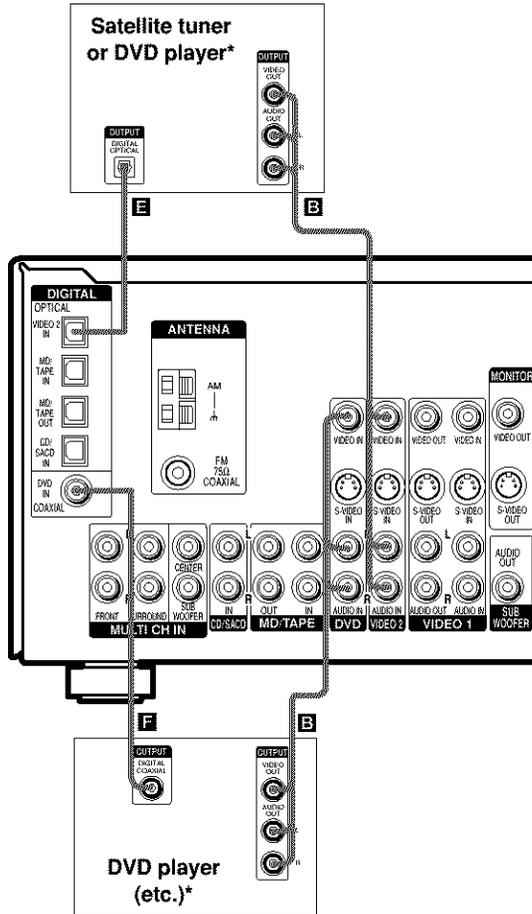
\* Make either coaxial or optical connections. We recommend making coaxial connections instead of optical connections.
