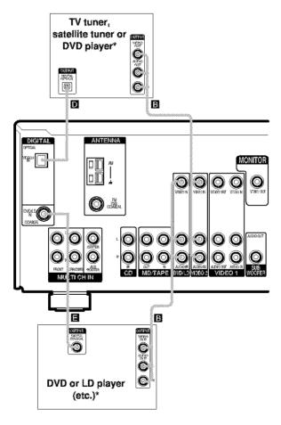
Make either coaxial or optical connections. We recommend making coaxial connections instead of optical connections.
