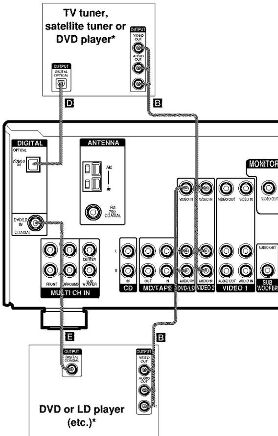
\* Make either coaxial or optical connections. We recommend making coaxial connections instead of optical connections.
