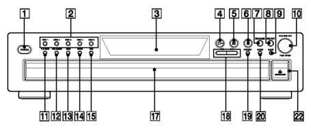
CHECK 20 (11, 12) CLEAR 9 (11, 12) DISC 1-5 2 (8, 9, 11) Disc compartment 17 (7) DISC SKIP 8 (7, 10, 12) Display 3 (9) EX-CHANGE 7 (10, 13) FADER 13 (12) PEAK SEARCH 12 (13)
