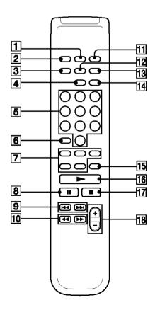
ANALOG OUT LEVEL +/-- 18 (6, 7) CHECK 12 (11, 12) CLEAR 13 (11, 12) CONTINUE 2 (8) DISC 1-5 7 (8, 9, 11) DISC SKIP 15 (7, 10, 12) FADER 14 (12) Number buttons 5 (9, 11) PROGRAM [11] (8) REPEAT 3 (8) SHUFFLE 1 (8) TIME 4 (9, 10)
