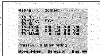
To unblock a rating, select it by moving the joystick up or down, then press  $\oplus$ . The indicator  $\boxplus$  changes into “-” and all “lower” ratings are unblocked.
