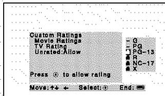
To unblock a rating, select it by moving the joystick up or down, then press  $\oplus$ . The indicator  $\text{🔒}$  changes into “-” and all “lower” ratings are unblocked.
