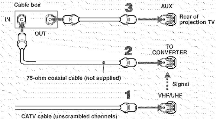
**⚠️** Pressing ANT on the remote control switches between the channels coming in through the cable box (scrambled) and those coming directly to the TV (unscrambled).
