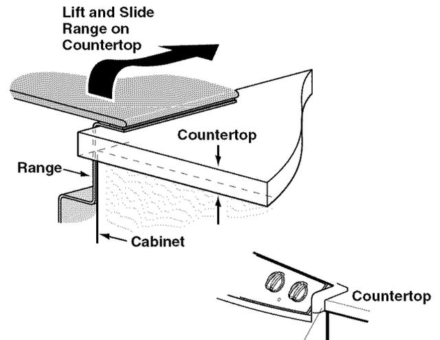
Make sure the edge of the countertop fits flush against the end of the Front Control Panel
