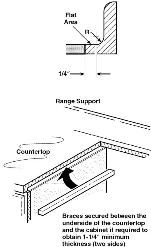
The Standard Installation of this Drop-In Range is to hang by the countertop on the side metal flanges under glass cooktop.
