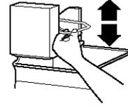
2. Install the interior water filter cartridge (on some models). The interior water filter mounting bracket is located in the upper corner of the fresh food compartment of the refrigerator.
