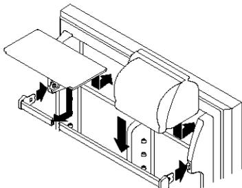
3. Adjust the utility compartment by lifting the front slightly and sliding it to the desired position. Lower the front to lock it into place.
