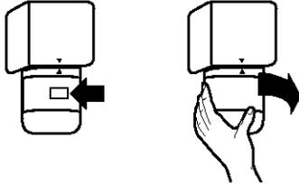
4. Line up the INSTALL mark on the water filter label with the indicator line that is molded into the filter mounting bracket cover. Push the cartridge into the filter mounting bracket. Twist the cartridge ¼ turn to the right to lock it into place. The REMOVE mark should be lined up with the indicator line located on the front cover.
