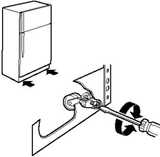
5. Open both doors again and check to make sure that they close as easily as you like. If not, tilt the refrigerator slightly more to the rear by turning both leveling screws to the right. It may take several more turns, and you should turn both leveling screws the same amount.
