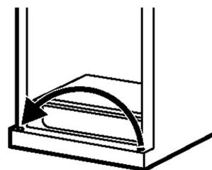
3.7 Take one of the screws removed in step 2 and start it in the outermost screw hole on the opposite side. Do not drive it all the way down—leave enough space under the screw head for thickness of shim and bracket.
