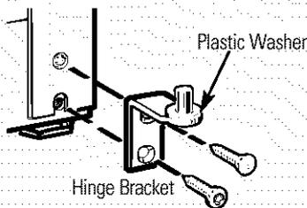
4.3 Interchange hinge (and the shim glued to it) and screws at top right with screws at top left of cabinet. **Do not tighten screws on hinge side at this time.**
