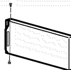
5.4.3 Remove the screw from the right top edge of the door and insert it into the handle screw hole on the left side.
