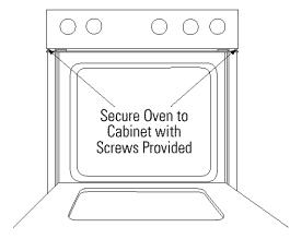
Secure oven to cabinet with screws provided. Single ovens use 2 screws, one on each side. Double ovens use 4 screws, 2 on each side.
