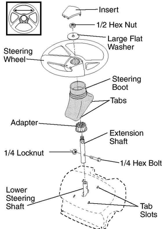
7. Snap steering wheel insert into center of steering wheel.
