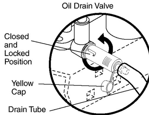
3. Unlock drain valve by pushing inward slightly and turning counterclockwise.
