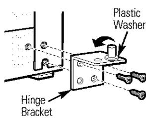
Models with a hinge bracket that has 4 screw holes. Switch the hinge pin to the opposite side of the bracket.
