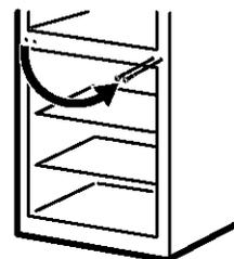
3.3 Remove the tape and tilt the door away from the cabinet. Lift the door from the pin in the bottom hinge bracket. (If the plastic washer sticks to the door bottom, put it back on the hinge.)
