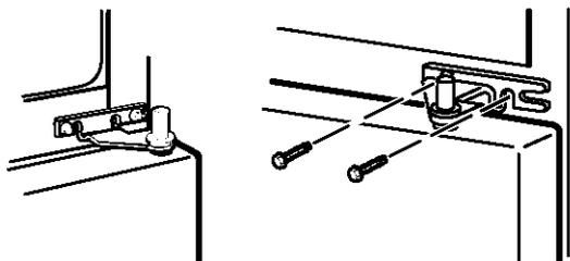
3.5 Transfer the two screws from the opposite side of the cabinet to the screw holes vacated by the center hinge removal.
