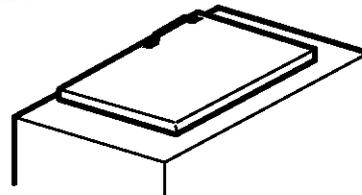
3.2 Using a 5/16" hex-head socket screwdriver and a 5/16" open-end wrench, remove the two screws holding the center hinge (and the shim glued to it) to the cabinet. Lift the center hinge to free its pin from the socket in the top of the door, and set hinge and screws aside. **Be careful not to lose the center hinge spacer and washer.**
