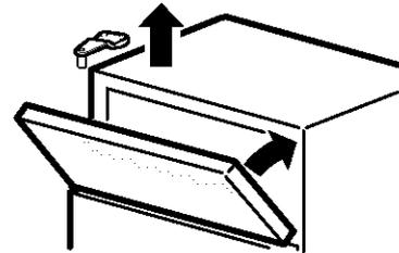
6.1.3 Tilt the door toward the cabinet. As the door is brought into position, slide the hinge under the head of the screw which earlier had been partly driven into the outermost hole. Insert the remaining screw, then tighten both screws securely.
