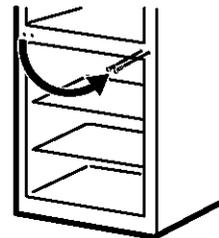
3.2 Using a 5/16" hex-head socket screwdriver and a 5/16" open-end wrench, remove the two screws holding the center hinge (and the shim glued to it) to the cabinet. Lift the center hinge to free its pin from the socket in the top of the door, and set hinge and screws aside. **Be careful not to lose the center hinge spacer and washer.**
