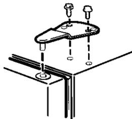
Installing the hinge on the right.
