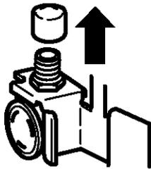
Place the compression nut and ferrule (sleeve) onto the end of the tubing as shown. On an approved plastic refrigerator tubing kit, the nuts are already assembled to the tubing.
