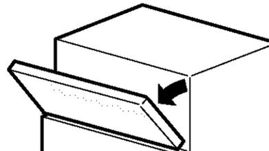
2.5 Set the door on a non-scratching surface with the outside up.
