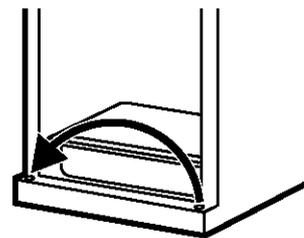
3.3 Remove the tape and tilt the door away from the cabinet. Lift the door from the pin in the bottom hinge bracket. (If the plastic washer sticks to the door bottom, put it back on the hinge.)
