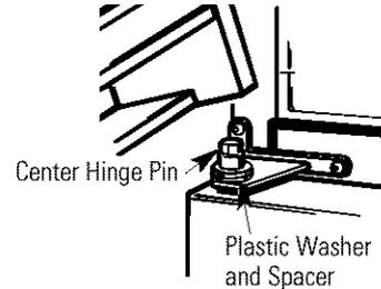
6.1.2 Insert the pin on the center hinge into the socket in the top of the door. Place the spacer, then the washer, on the hinge pin. **NOTE:** The center hinge must be turned over as shown when mounted on the left side.
