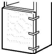
3.5 Transfer the two screws from the opposite side of the cabinet to the screw holes vacated by the center hinge removal.
