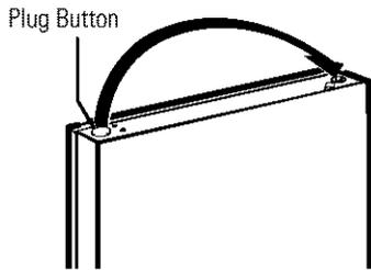
5.1.5 Pull the plug button from the front of the door and transfer it to the opposite side.
