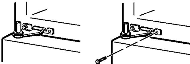
6.2.3 Make sure the door is slightly above the top of the cabinet and the gap between the doors is even across the front. Tighten the top hinge screws. Do not overtighten these screws—tighten them until they are just snug, then turn them another one-half turn.
