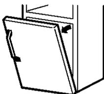
3.7 Take one of the screws removed in step 2 and start it in the outermost screw hole on the opposite side. Do not drive it all the way down—leave enough space under the screw head for thickness of shim and bracket.
