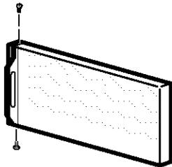
5.4.3 Remove the screw from the right top edge of the door and insert it into the handle screw hole on the left side.
