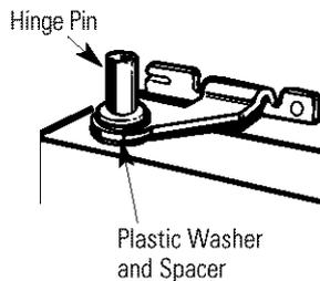
6.2.2 Tilt the door toward the cabinet, lifting the top hinge so the pin fits into the socket on the top of the door.
