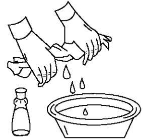
Soak the wiping cloth in cool, clean water and mild detergent. Then ring the cloth out before using.
