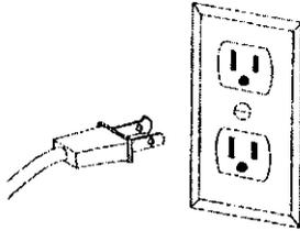
To reduce the risk of electrical shock, this saw has a polarized plug (one blade is wider than the other). This plug will fit in a polarized outlet only one way. If the plug does not fit fully in the outlet, reverse the plug. If it still does not fit, contact a qualified electrician to install the proper outlet. Do not change the plug in any way.
