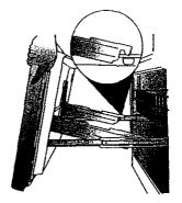
With drawer pulled out to full extension, insert lower basket by aligning tabs on both side of lower basket with notches in rail assembly.
