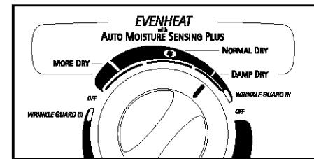
Some fabrics will shrink if dried in a clothes dryer. Selecting DAMP DRY gives you the benefit of electronic moisture sensing. Clothes are dried with heat for a brief time so most of the moisture is removed. However, the drying cycle stops while the clothes are still damp to prevent overdrying. As a result, fabrics retain the proper amount of moisture so they will not shrink.
