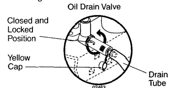
3. Unlock drain valve by pushing inward slightly and turning counterclockwise.
