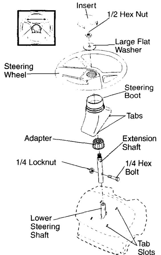
7. Snap steering wheel insert into center of steering wheel.
