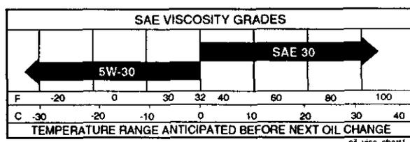
**NOTE:** Although multi-viscosity oils (5W30, 10W30 etc.) improve starting in cold weather, these multi-viscosity oils will result in increased oil consumption when used above 32°F.
