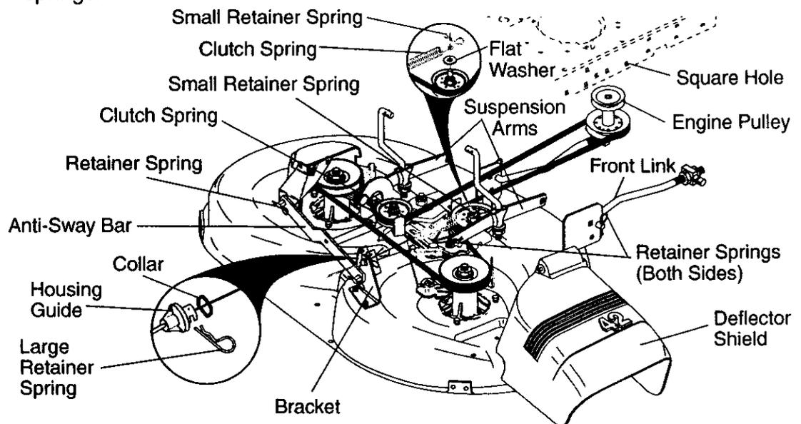
5. Connect suspension arms to rear deck brackets and secure with retainer springs.
