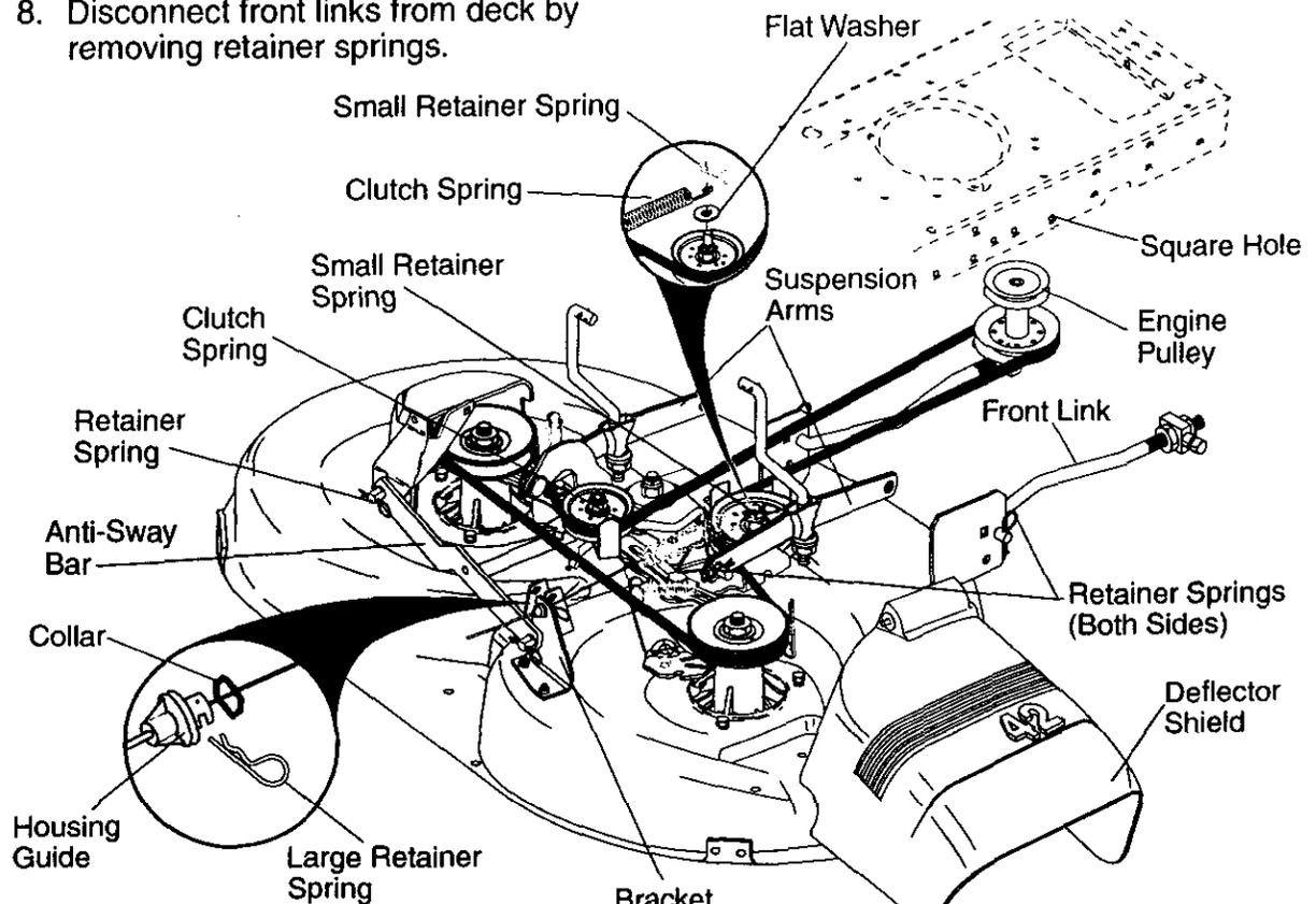
7. Push clutch cable housing guide into bracket, slide collar onto guide and secure with large retainer spring.
