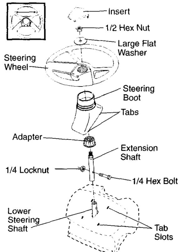
7. Snap steering wheel insert into center of steering wheel.
