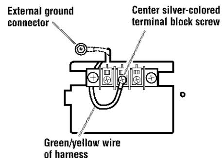
5. Connect neutral grounding wire and the neutral wire (white or center) of direct wire cable under the center screw of terminal block.
