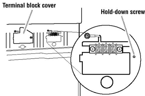
3. Attach a 3/8-inch, U.L.-listed, strain relief to the hole below terminal block opening. Strain relief should have a tight fit with dryer cabinet and be in a horizontal position. Put the power supply cord through the strain relief.
