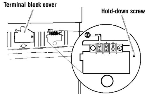
4. Remove the center terminal block screw. Remove the neutral grounding wire (green/yellow wire) from external grounding screw.
