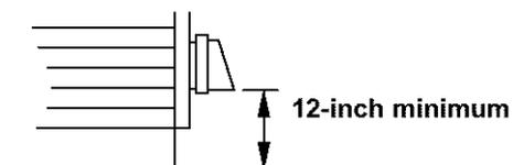
A 4-inch outlet exhaust hood is preferred. However, a 2½ inch outlet exhaust hood may be used. A 2½ inch outlet creates a greater back pressure than other hood types. Smaller hoods increase drying time. For
