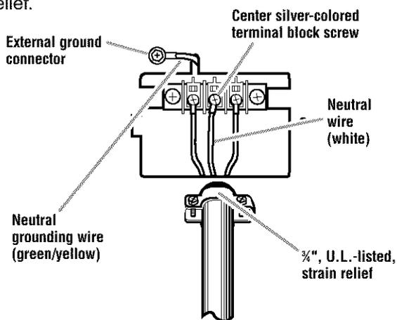
4. Loosen or remove terminal block screws. Connect the neutral wire (white or center) of power supply cord under the center screw of the terminal block.
