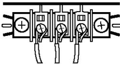
7. Connect the other two wires to outer terminal block screws. Use the same method described in Step 6.
