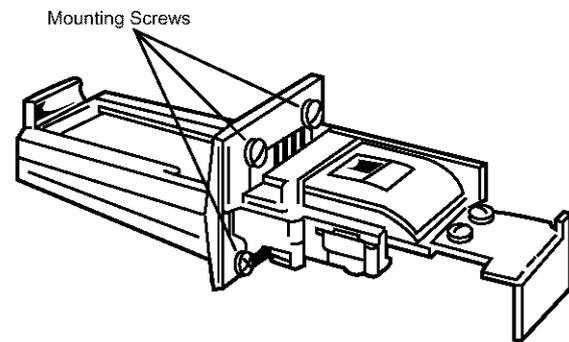
3. Insert the coin slide mechanism through the opening to the left of the control panel. You may have to loosen four mounting screws for proper fit.
