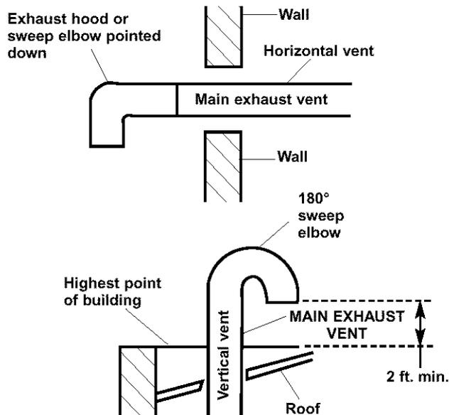
**NOTE: Do not** install screening or cap over end of vent.
