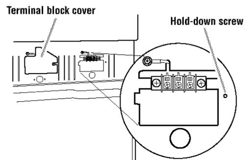
3. Attach a 3/4-inch, U.L.-listed, strain relief to the hole below terminal block opening. Strain relief should have a tight fit with dryer cabinet and be in a horizontal position. Put the direct wire cable through the strain relief.
