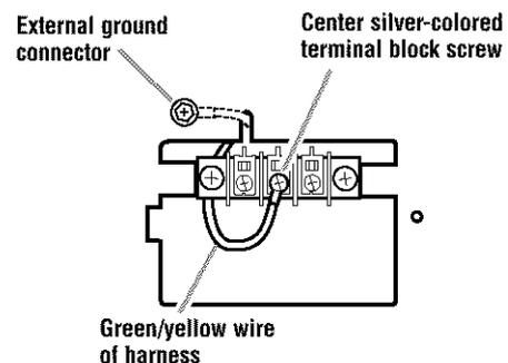
5. Connect neutral grounding wire from machine and the neutral wire (white) of power supply cord under the center screw of terminal block.
