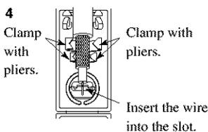
Insert the cable wire into the slot, and clamp it with pliers.
