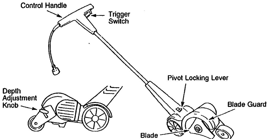
The **TRIGGER SWITCH** is used to activate the motor.
