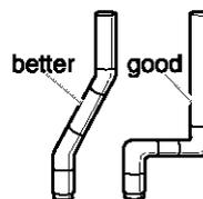
4. Use clamps to seal all joints. Do not use duct tape, screws or other fastening devices that extend into the interior of the vent to secure vent.
