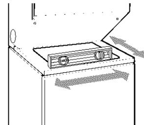
2. If the laundry center is not level, prop up the front with a wood block and adjust the feet up or down as necessary. Remove wood block and lower laundry center. Repeat this step until the laundry center is level.
