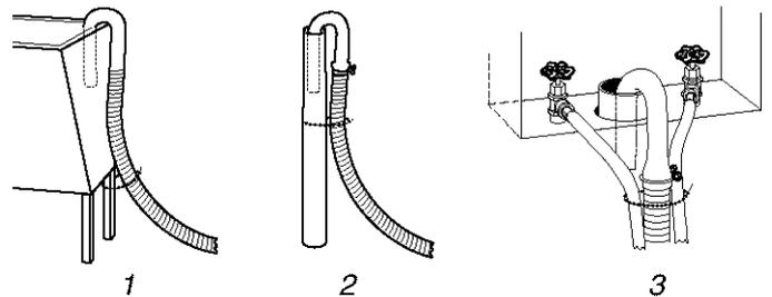
If the water faucets and the drain standpipe are recessed, put the hooked end of the drain hose in the standpipe. Tightly wrap the plastic strap around the water inlet hoses and the drain hose (3 above).
