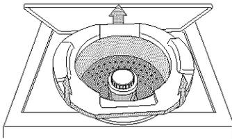
**NOTE:** Keep the foam ring and use it when transporting your laundry center. This packing material is used to keep the washer tub stable during transport.
