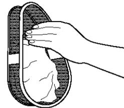
4. Put the lint screen and cover back together and push firmly back into place.
