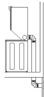
Terminate the exhaust vent outside. The exhaust vent must not terminate beneath the mobile home and must not be connected to any other duct, vent or chimney.
