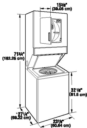
\*Most installations require a minimum 5½ in. (14 cm) clearance behind the dryer for the exhaust vent with elbow. See "Venting Requirements."
