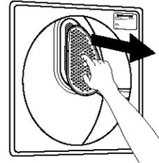
2. Separate the cover and the screen by squeezing the screen and pulling on the cover at the same time.
