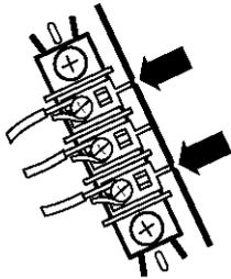
4. Tighten strain relief screws.
