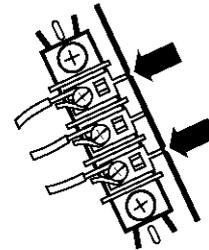
6. Tighten strain relief screws.
