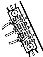
1. Remove center terminal block screw.
