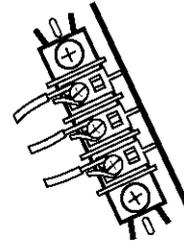
1. Loosen or remove center terminal block screw.
