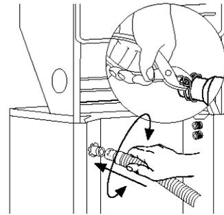
4. Place clamp over the area marked "CLAMP." Release clamp.
