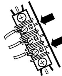
4. Tighten strain relief screws.
