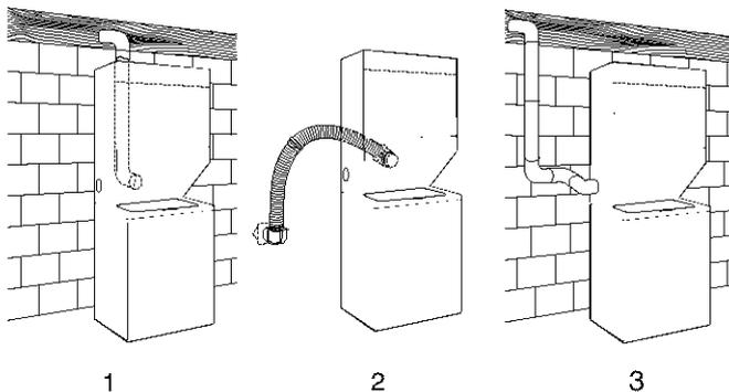
1. Standard rear offset exhaust installation
