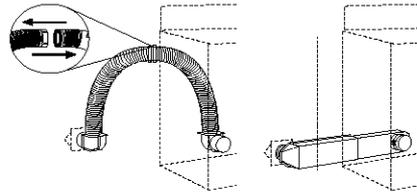
1. Over-The-Top installation (also available with one offset elbow)
