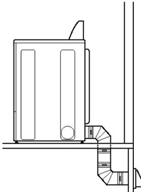
Terminate the exhaust vent outside. The exhaust vent must not terminate beneath the mobile home and must not be connected to any other duct, vent or chimney.
