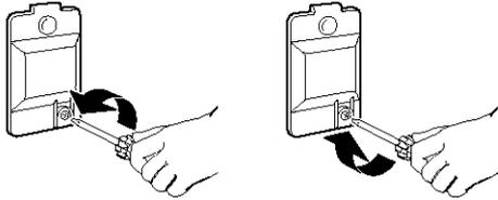
**STEP 3.** Turn bulb counterclockwise. Replace the bulb with a 10-watt appliance bulb only. Replace the cover and secure with the screw.
