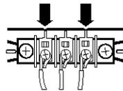
6. Tighten strain relief screws.
