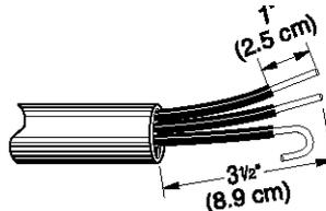
When connecting to the terminal block, place the hooked end of the wire under the screw of the terminal block (hook facing right), squeeze hooked end together and tighten screw.
