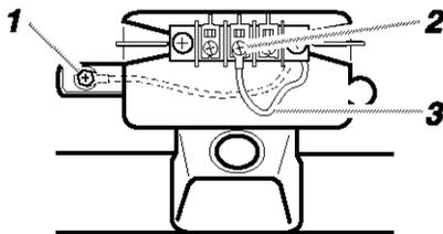
1. External ground connector - Dotted line shows position of NEUTRAL ground wire before being moved to center terminal block screw
