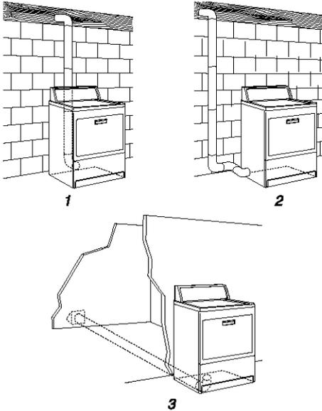
1. Standard rear offset exhaust installation
