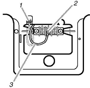
1. External ground connector - Dotted line shows position of NEUTRAL ground wire before being moved to center terminal block screw
