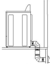
the interior of the vent to secure vent. Terminate the exhaust vent outside. The exhaust vent must not terminate beneath the mobile home and must not be connected to any other duct, vent or chimney.
