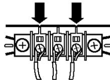
6. Tighten strain relief screws.
