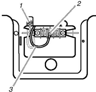
1. External ground connector - Dotted line shows position of NEUTRAL ground wire before being moved to center terminal block screw
