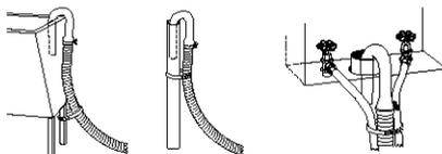
If the washer faucets and the drain standpipe are recessed, put the hooked end of the drain hose in the standpipe. Tightly wrap the tie strap around the water inlet hoses and the drain hose.
