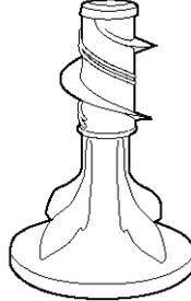
The best cleaning action in your washer takes place at the bottom where the agitator vanes move back and forth to flex the fabric, loosening the soil. To get all your clothes down to the bottom of the washer, the upper portion of the agitator has uniquely designed, spiral vanes to help push the clothes that are on top down to the bottom. This spiraling action displaces the clothes that are on the bottom with a "roll-over" motion.
