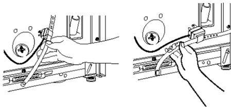
2. Pull firmly to remove the end of the shipping strap that remains pinned to the back of the washer. This will release the rear self-leveling feet.
