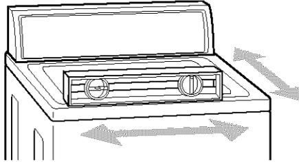
**STEP 7.** If washer is not level, prop up the front of the washer and adjust the legs up or down as necessary. Lower washer and reset self-adjusting rear legs (as in Step 6). Repeat Step 7 until the washer is level.
