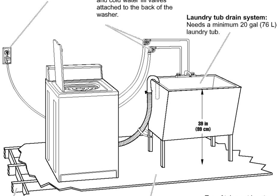
**Support:** Floor must be sturdy enough to support a total weight of 315 lbs (143 kg) (including washer, water, and load weight).
