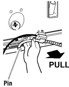
**STEP 3.** Cut the shipping strap about 16 in (40 cm) from plug end. Look for the words "CUT HERE." Discard end with the cotter pins. **Slide remainder of shipping strap from the electrical plug.** You will use this to secure the drain hose.
