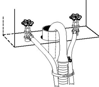
**STEP 2.** Locate the remaining piece of shipping strap (not the end with the cotter pins) from STEP 3 of "REMOVE SHIPPING STRAP." Use it to wrap the drain hose together with the laundry tub or standpipe. Push fastener into the nearest hole in the shipping strap.
