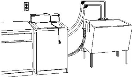
If the water faucets and drain standpipe are recessed, put hooked end of drain hose in standpipe. Tightly wrap the shipping strap around the drain hose and water inlet hoses (not the handles or stems). Push fastener into the nearest hole in the shipping strap.
