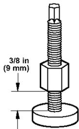
**STEP 3.** Screw leg into washer base by hand until nut reaches washer base. Repeat for other leg.
