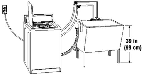
Standpipe Drain System (p. 13)
